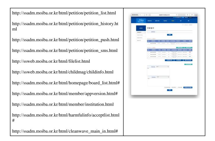
These addresses appear to demonstrate at least an initial version of the administrative interfaces for the Smart Sheriff application that is used to manage user accounts, restrict access to sites, and display a log of user interactions for all users. Given the authentication issues noted previously, these pages may leak information on vulnerable administrative APIs.
