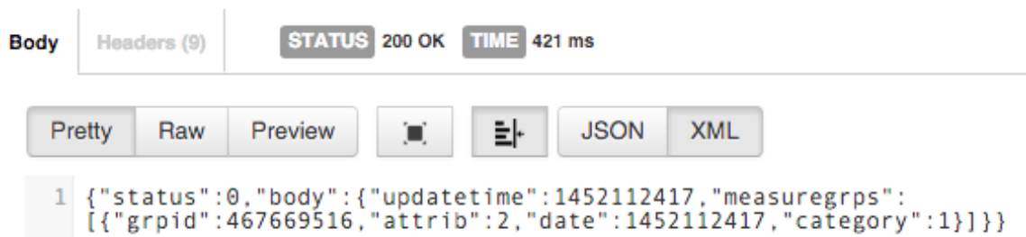
Figure 8: The Withings server responding to the HTTP request containing a falsified heart rate measurement. “Status: 0” indicates the server accepted the data. Other information present include the time at which the server accepted the request and the time associated with the heart rate measurement.
