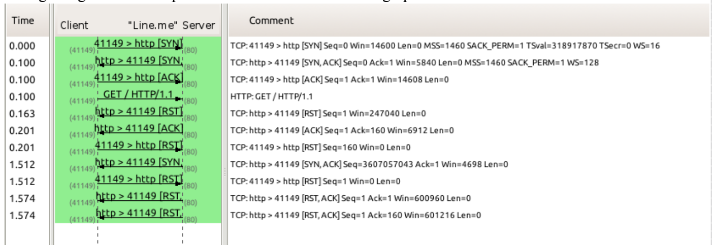
Figure 3 – TCP Flow graph of an injected RST response for line.me
