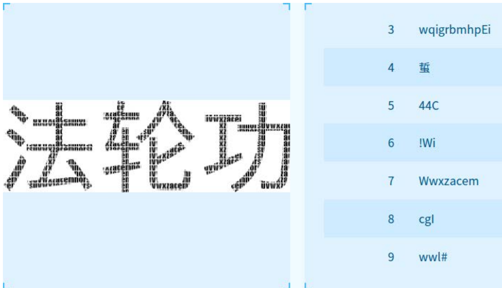
Figure 5: Output of Tencent Cloud OCR when uploading the Falun Gong image from Figure 4. The filter finds the constituent letters making up the characters, as well as other erroneous symbols, but not the characters 法轮功 themselves.
