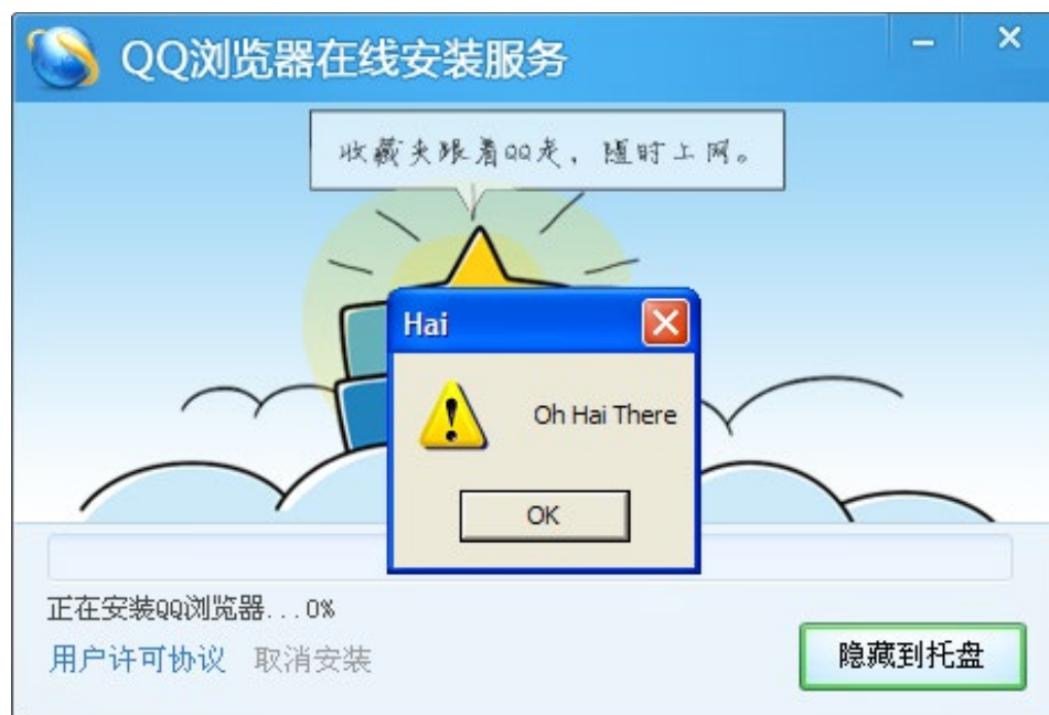
Figure 3: Example man-in-the-middle attack on QQ Browser's self-updater by first injecting a vulnerable Web installer and then injecting our arbitrary program. A benign program that displays "Oh Hai There" was used as the payload, but any arbitrary program such as spyware or malware could be injected.
