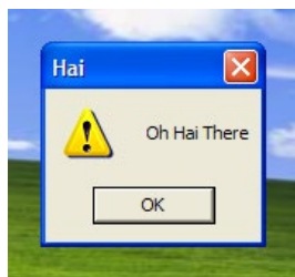
Figure 1: Example man-in-the-middle attack on UC Browser’s self-updater. When the updater silently runs in the background, we inject our own update that contains an arbitrary program that is then executed with Windows SYSTEM privileges. Our benign program displays “Oh Hai There,” but any arbitrary program such as malware or spyware could have been injected.
